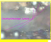
Although the equipment particle concentration (EPC) of 269 is well within acceptable limits for this type of equipment, analytical results show a high concentration of Ferrous metal wear particles. These metal particles are from the LTC mounting hardware. The movement of this hardware has resulted in the electrical discharge to surrounding components and contacts. This image displays the Techtites or Spheres (i.e. the Sparks) from electrical discharge.
